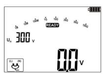
After inserting WS-04 / WS-11 into the socket, the screen displays a message indicating the detection of the adapter.
