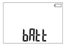
Batteries / rechargeable batteries fully discharged.
