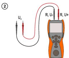
Connect the meter to a voltage source.
